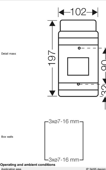
IP 54/65 design: Suitable for indoor installation and outdoor installation, protected against weather influences IP 40/41 design: Suitable for installation in dry indoor areas However, pay attention to the climatic effects on the installed equipment, for example, high or low ambient temperatures or formation of condensed water see technical information
